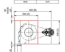
FLAMESHIELD FS120 JM HEAD BOX SIZE B: 400 x 400mm MOTOR ENDPLATE B: 600 x 400mm
