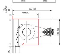
FLAMESHIELD FS120 JM HEAD BOX SIZE B: 450 x 450mm MOTOR ENDPLATE B: 650 x 450mm
