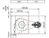
FLAMESHIELD FS120 JM HEAD BOX SIZE B: 400 x 400mm MOTOR ENDPLATE B: 600 x 400mm
